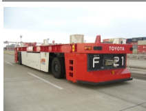
76 12GB30904 Automated Guided Vehicle System [TOYOTA Automated Guided Container Transport System] This system is constructed of unmanned vehicles carrying containers and the software that controls this operation.
